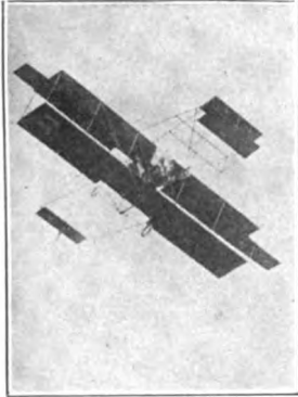
Hamilton's machine patterned after the Curtiss type and equipped with a Christie motor of 110 indicated horsepower. The motor was not ready and the machine seldom flew
